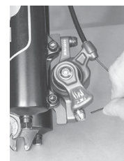
Step C-7 Stringing Cable
